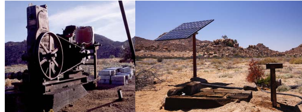
The old diesel pump and the new solar pump
